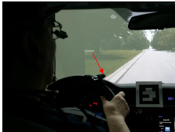
Figure 8. Over the shoulder view of screen with laser (red arrow) at top of steering wheel during driver performance testing of the 2014 Toyota Corolla infotainment system
