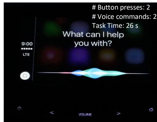
Figure 13. CarPlay (paired CUE and iPhone). Destination entry with Siri voice system with auditory input to driver from car speakers, showing redundant visual display on vehicle screen with moving colored images at bottom
