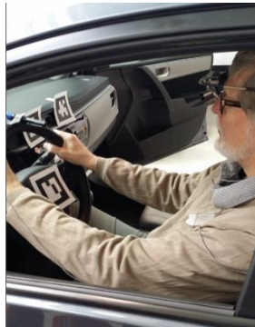
Figure 7. Test set-up for driver performance testing of 2014 Toyota Corolla infotainment system. See Seaman et al. (2016) for further set-up and task details
